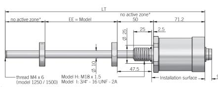
$^{\star} = 55$  mm up to stroke 1000 mm, from 1250 mm consider 60 mm due to M4 threaded hole
