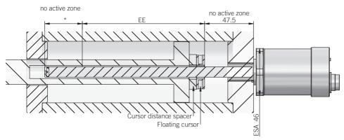
\* = 55 mm up to stroke 1000 mm, from 1250 mm consider 60 mm due to M4 threaded hole
