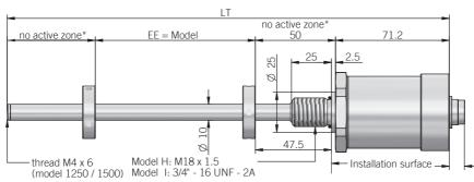
$^{\ast} = 55$  mm up to stroke 1000 mm, from 1250 mm consider 60 mm due to M4 threaded hole
